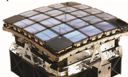
**Above:** *Kepler's* image sensor array, which is curved to account for Petzval field curvature. **Right:** Sky diagram of *Kepler's* investigated area. (Credit: Wikimedia Commons)
