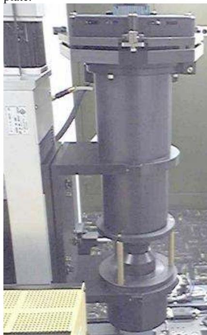
The camera has 4096 x 4096 pixels, 11 microns square with 12-bit accuracy at 2300 dpi. Donated by Photon Dynamics. Readout is via the CameraLink interface at close 1.8 Gbit/sec. The 32MB image is read out in 140 milliseconds. The lens is a double telecentric lens, which preserves 1:1 scaling even when out of focus. The camera is mounted on a screw drive stage, which can set focus accurately to 5 microns. The camera and lens assembly is approximately 18 inches long. The next challenge was to
