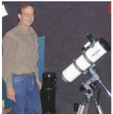
swapped the front lens from a Stellarvue scope for the optics in a Magrez scope and ended up with sharp, low-color optics and a smooth focuser.
